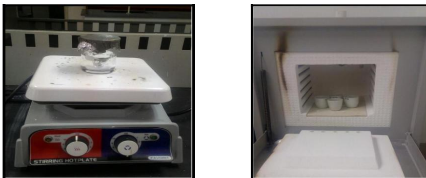
(a) (b) FIGURE 1. Procedure of (a) stirring process to obtain clear solution and (b) annealing process
